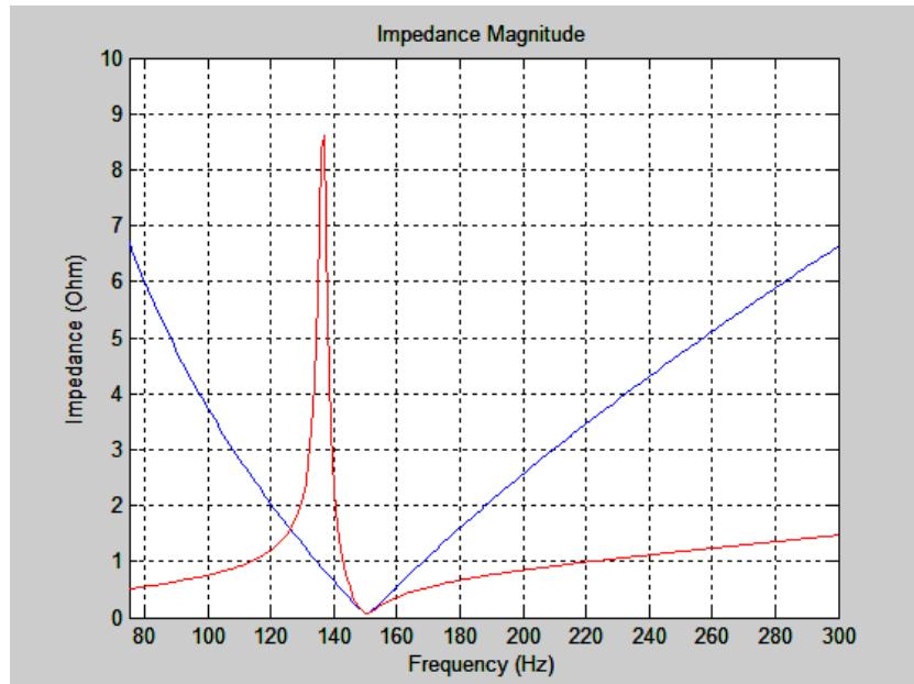
In some cases of wrong design or due to ageing of filter equipment, the latter especially causing a capacitance drop, the parallel resonance frequency changes in such a way that it may coincide with a current harmonic frequency injected by the load. This will cause overvoltages and overcurrents in the system equipment, leading to failure; and in some cases together with catastrophic damage.
